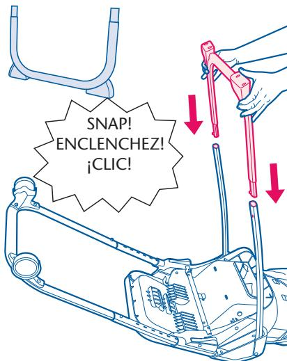
Insert other "U" tube into the rear tubes until they snap into place.
